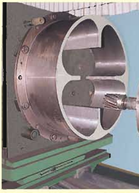
Machining of 6.5MW DCB Coupling, outer member 1.2 metre in dia
