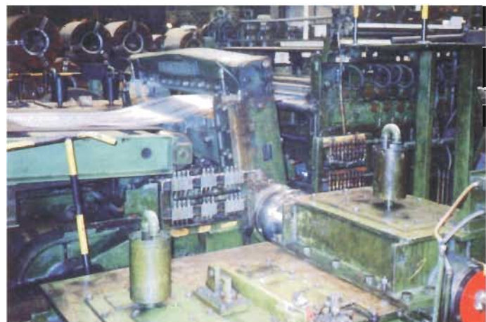
PM18 and Pm27 coupling on a Halden-Robertson type 56 flying shear in Portugal.
